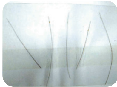
Attach the hair to be investigated on mounting paper using cellophane tape
